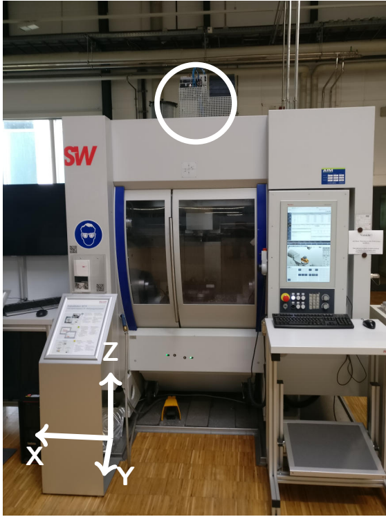
(a) CNC milling machine. Circle: Position of the additionally applied vibration sensor on top of the machine.
