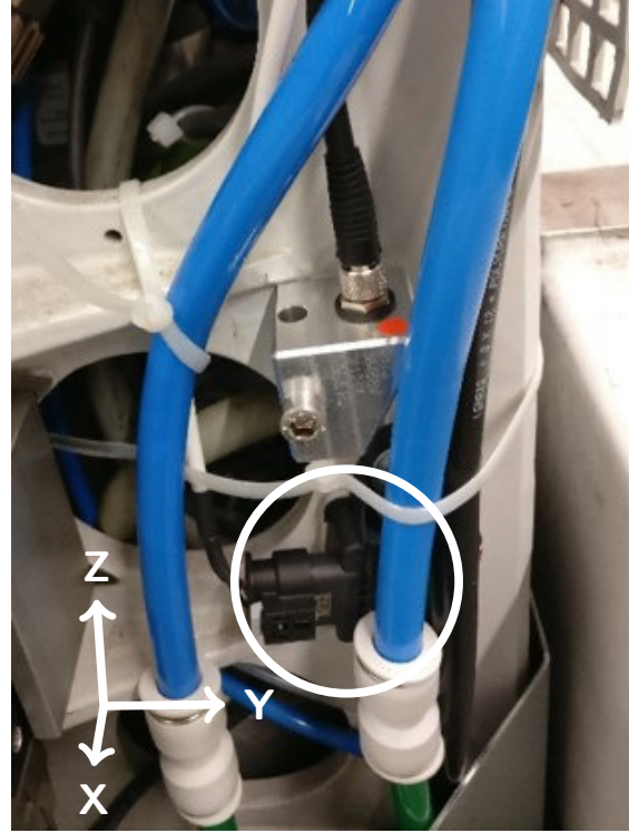
(b) Closer view on the mounting position of the vibration sensor. Compared to Figure 2a, the z-axis is rotated by 90 degrees.
